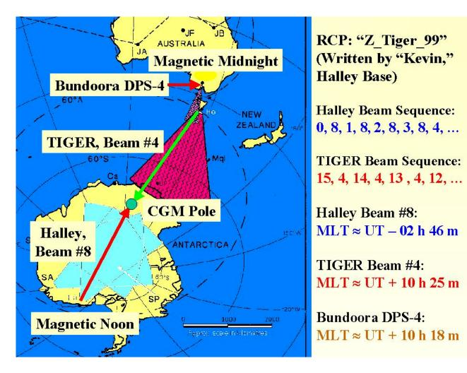
**Figure 1:** Layout of the experiment designed to measure the time delay between the start of an IMF driven convection change in the dayside ionosphere and its manifestation in the high-latitude nightside ionosphere, and the subsequent penetration of magnetospheric convection fields into the plasmasphere.
